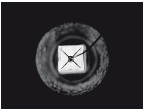
Fig. 7.17 Image of LED chip light emission
