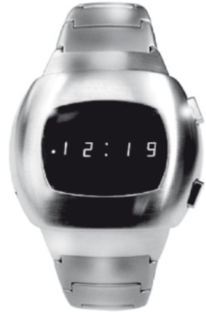
Fig. 4.1 Digital wristwatch implementing red LED display
