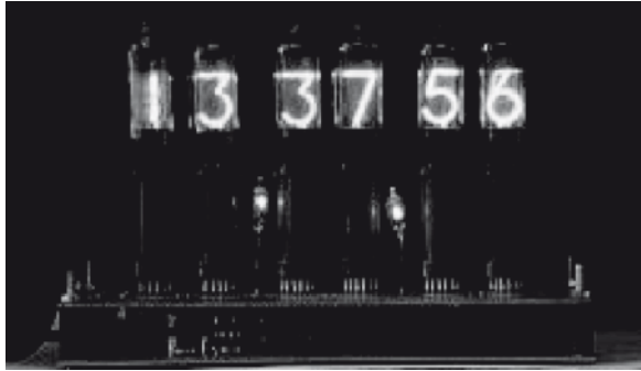
Fig. 4.3 Watch based on nixie display
