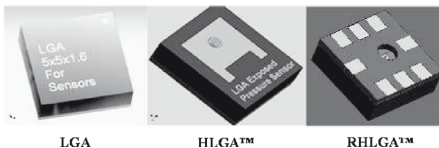
Fig. 5.34 Three possible solutions for MEMS package. LGA for hermetic products. HLGA™ and RHLGA™ for non-hermetic ones
