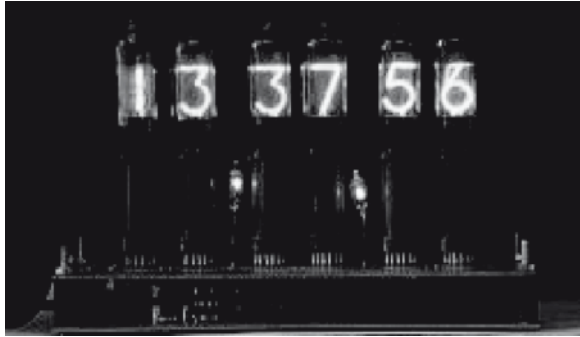
Fig. 4.3 Watch based on nixie display
