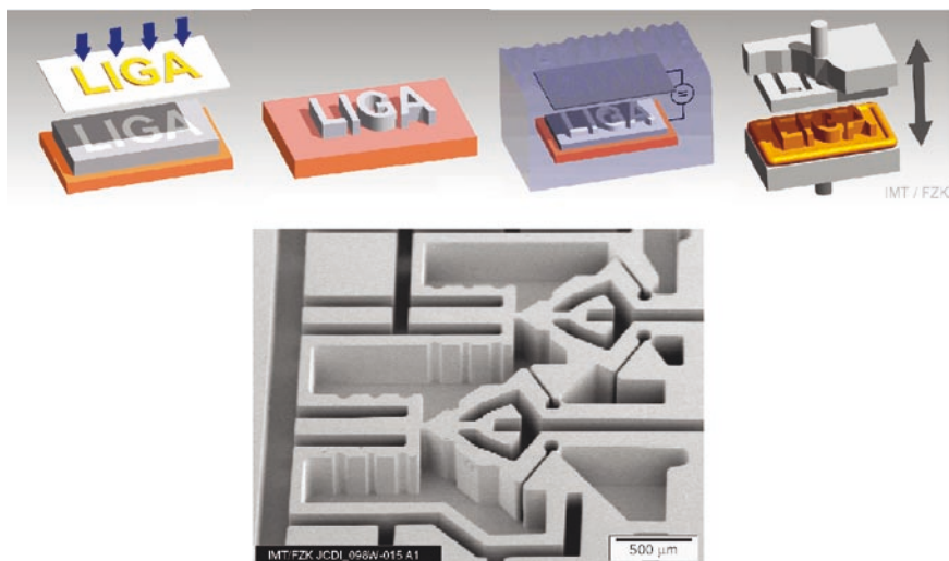
Fig. 5.24 X-ray LIGA: Process principle for the fabrication of the metal template used for polymer injection. Top row from left to right: Exposure, structure after development, electroplating, and replication. The bottom picture shows an example of a fabricated structure used in a FTIR spectrometer. Images courtesy of the Institute for Microstructure Technology (IMT), Karlsruhe Institute of Technology
