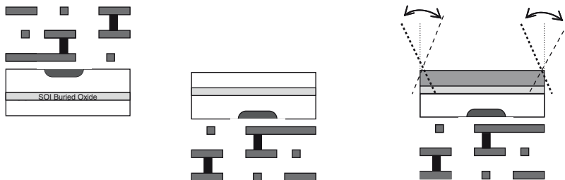
Fig. 8.12 Back side technique to overcome the light path screening through interconnects for large optical aperture (low f\# )
