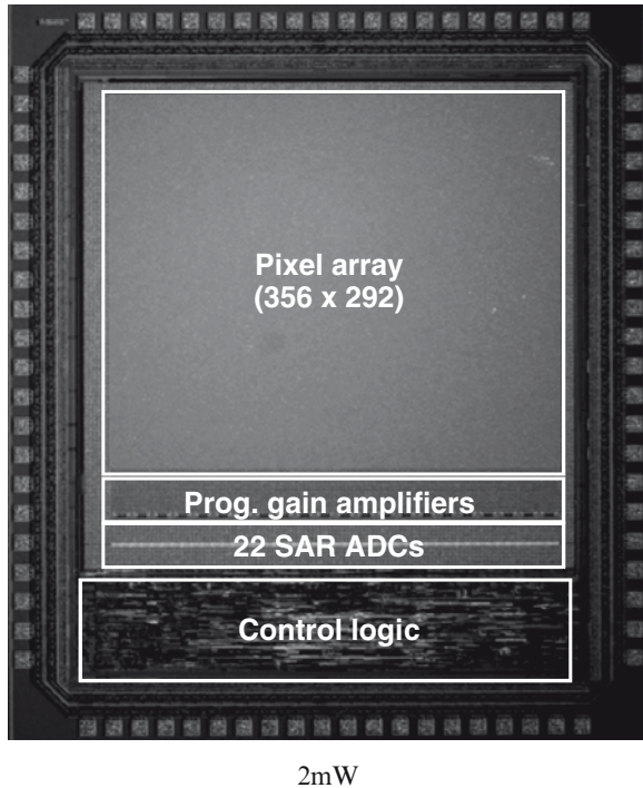
Fig. 8.8 Micrograph of a digital single-chip camera with a power consumption of less than 2 mW
