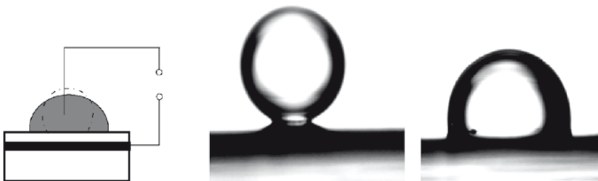
Fig. 6.3 EWOD principle and pictures of a droplet without and with EWOD actuation
