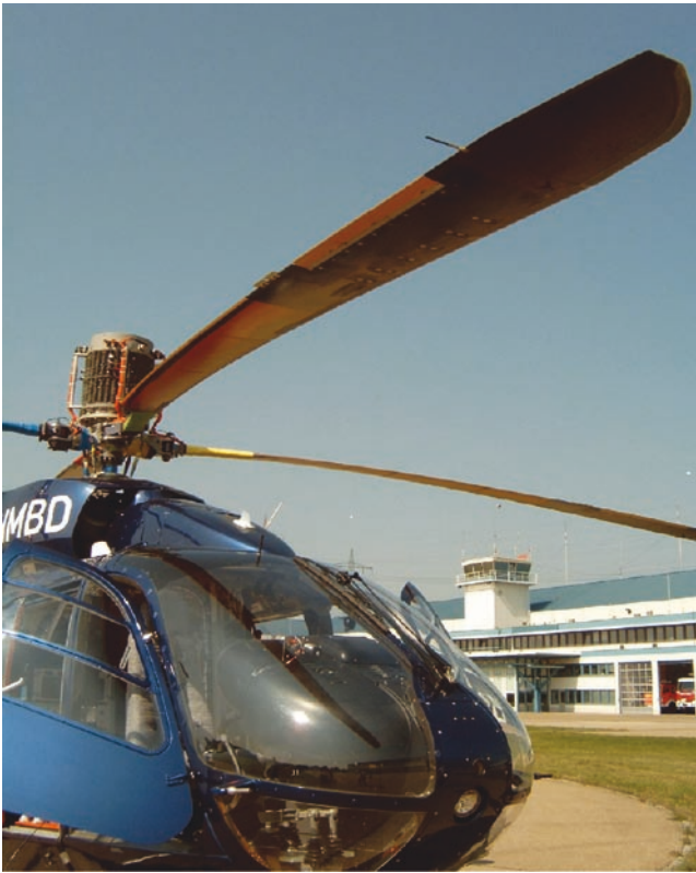
Fig. 2.9 Eurocopter with adaptive rotor blades for efficient operation, low noise and low vibration (by courtesy of EADS Deutschland GmbH)
