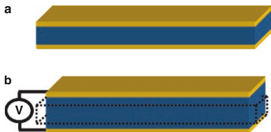
Fig. 5.2 Capacitor structure for piezoelectric sensor/actuator. The piezoelectric material is shown in blue and the metal electrodes in yellow
