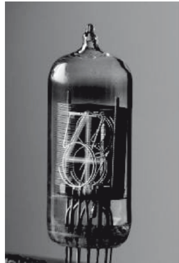
Fig. 4.2 An example of NIXIE tube with numerical digits
