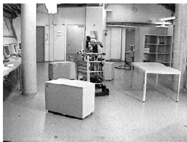
Fig. 11.2 Exploration system Marvin using binocular stereo.
