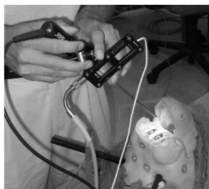
Fig. 11.15 Experimental setup for the validation of the accuracy of the endoscope navigation in a porcine cadaver head.
