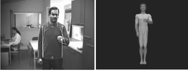
Fig. 4.2 Illustration of the performance of the markerless human motion capture system. Left: projection of the estimated configuration into the left camera image. Right: 3D visualization of the estimated configuration with an articulated human model.
