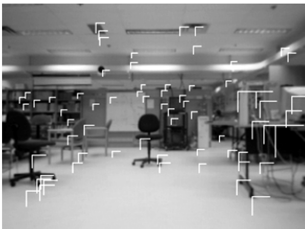
Fig. 10.1 SIFT features found by our stereo-equipped robot. SIFT features in the three stereo images are matched; horizontal and vertical lines indicate the horizontal and vertical disparities respectively (from [16]).
