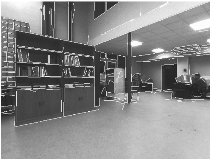
Fig. 9.6 A typical result of a line segment extraction algorithm: some segments are artifacts, and others are longer or smaller than the actual line in the environment.
