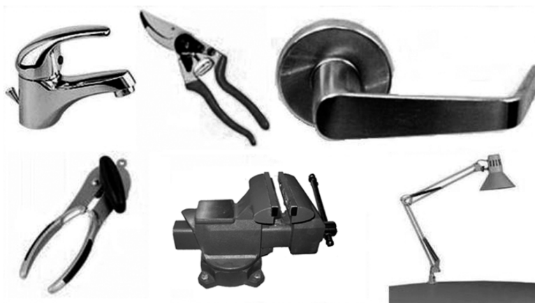
Fig. 2.1 Objects that possess inherent degrees of freedom; these degrees of freedom cannot be extracted from visual information alone, they have to be discovered through physical interaction
