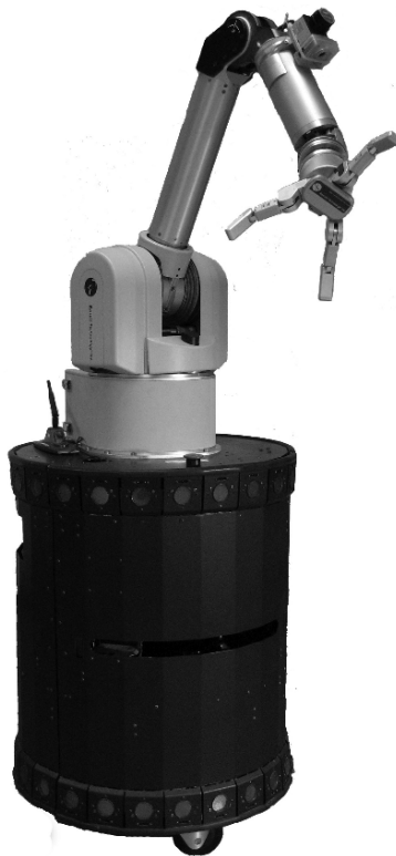
Fig. 2.2 UMan (UMass Mobile Manipulator) consists of a holonomic mobile base with three degrees of freedom, a seven-degrees-of-freedom Barrett Technologies manipulator arm, and a four-degrees-of-freedom Barrett hand.
