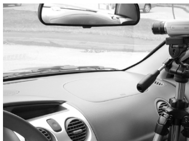
Fig. 11.5 Large baseline can easily be constructed utilizing the motion of the vehicle with monocular systems.
