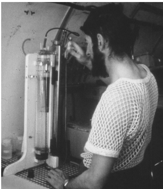
Figure 3. The author, inside the Silver Hut, using the Lloyd-Haldane apparatus to analyse alveolar gas samples for oxygen and carbon dioxide after a control of breathing experiment.
