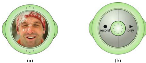
Fig. 6.4 Magnets that allow items on fridge surfaces to be annotated: (a) indicates who created it and (b) allows voice recordings
