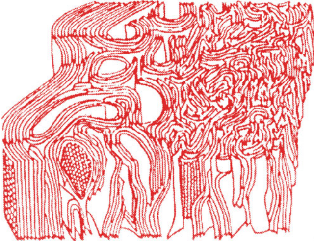
Fig. 2.22 Three-dimensional representation of PAN-based carbon fiber [from Bennett and Johnson (1978), used with permission]
