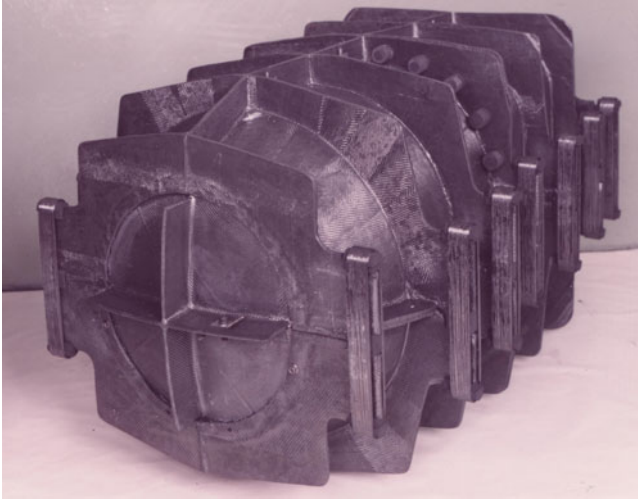
Fig. 8.9 A mold made of carbon/carbon composite (courtesy of SIGRI)
