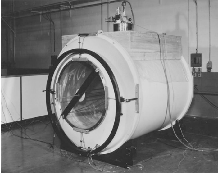
Fig. 9.15 A magnetic resonance imaging system for clinical diagnostics, under preparation (courtesy of Oxford-Airco)
