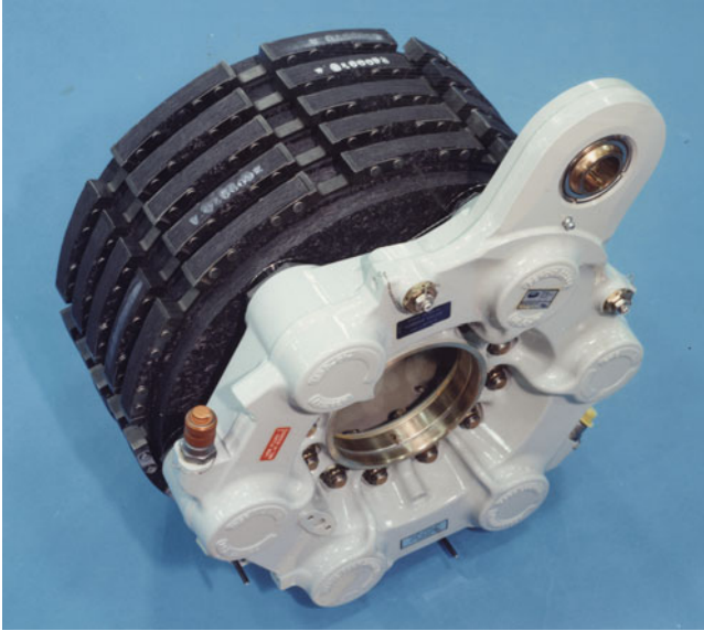
Fig. 8.8 A carbon/carbon brake assembly that is used on a Boeing 767 airplane (courtesy of Allied-Signal Corp.)
