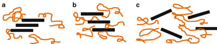
Fig. 15.1 Three different morphologies of platelets ( black ) dispersed in a polymeric matrix: (a) immiscible, (b) intercalated, and (c) miscible. Note the increased spacing between sheets in (b)
