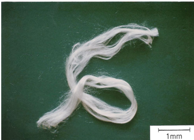
Fig. 2.5 Continuous glass fibers (cut from a spool) obtained by the sol-gel technique [from Sakka (1985), used with permission]
