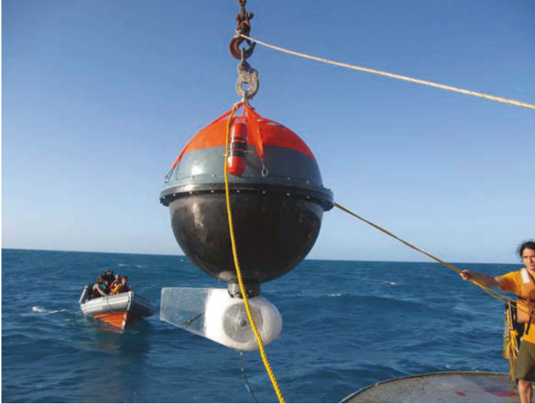
Figure 1.34: The instrumented buoy for the wave-powered station-keeping Buoy (WPSB)
