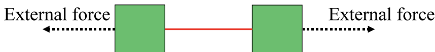
Figure 1.6: Two rigid bodies and a single string that do not constitute a tensegrity configuration
