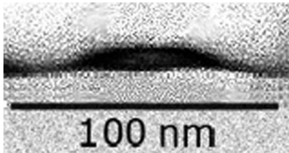
Fig. 6.2 Transmission electron microscopy image of a single InGaAs/GaAs quantum dot
