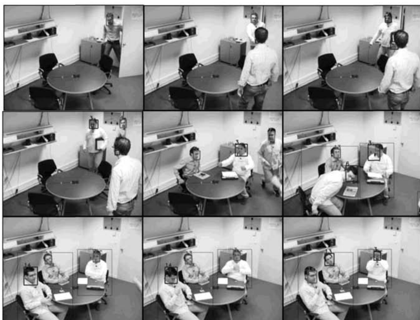
Fig. 1. Typical performance of the AIT face tracker. Detections of the three cascades of simple classifiers are marked in red, while faces being tracked by the CAM-Shift tracker are marked in blue. Notice that the latter are occluded or tilted faces
