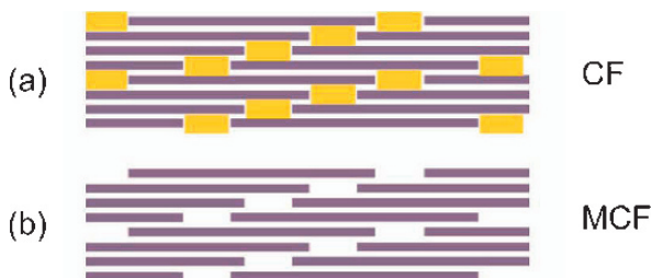
Fig. 8.34 Overview of the two structures considered here; subplot (a) shows a CF and subplot (b) shows a MCF (original study reported in Buehler 2007). The structures are loading in uniaxial tension along the axis of the TC molecules
