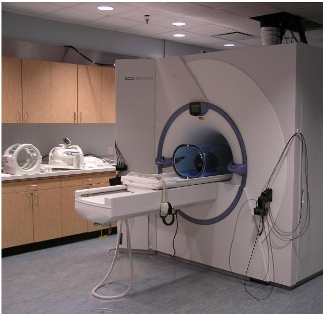
Fig. 9.14. Typical MRI scanner. This scanner has a “closed-bore” design, meaning that the patient lies on a bed within a cylindrical bore. The tank on the bed is a test pattern used for calibration of the scanner during maintenance. This particular scanner is used extensively for functional brain imaging, so there are many cables and sensors for providing audiovisual stimulation and feedback to the patient during imaging. Specialty coils for head imaging are seen on the shelf to the left of the scanner
