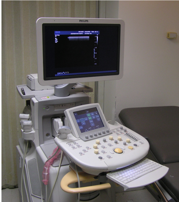
Fig. 9.15. Photograph of a medical ultrasound imaging system. As with most ultrasound units, the entire system is on a wheeled cart, so it can easily be moved around the hospital. The integrated system includes a keyboard, additional imaging controls, a monitor for viewing the images, and a small printer for hardcopy output. Different ultrasound probes and other supplies for imaging can also be stored on the cart
