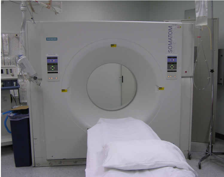
Fig. 9.5. Photograph of a CT scanner used for image-guided interventions. This scanner has a CT fluoroscopy mode for acquiring images in near real time (approximately 6 frames/s), which enables CT-guided interventions
