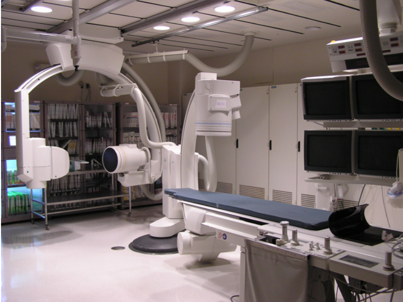
Fig. 9.3. Fluoroscopy system. The patient table is shown in the foreground, and viewing monitors for the fluoroscopy images are visible in the upper right of the photo. One C-arm is mounted on a rotating floor plate that allows it to move in and out from the patient table, and the other is mounted on rails in the ceiling that allow it to move around the room. The C-arm closest to the table is oriented so that the x-ray generator is below the table and the image intensifier is above the table
