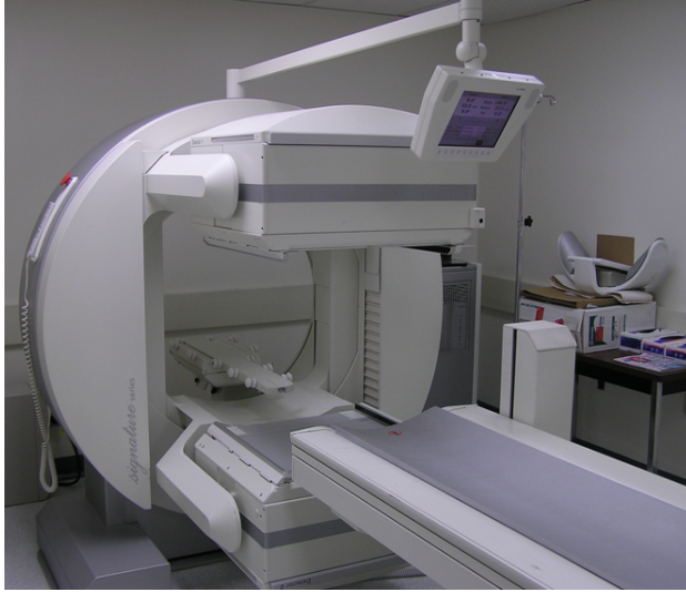
Fig. 9.12. Photograph of a SPET scanner. This SPET scanner shown in the photograph has two imaging cameras, one above the patient bed and one below the patient. The cameras are mounted on a gantry that allows them to rotate around the patient in order to collect projection data from multiple angles
