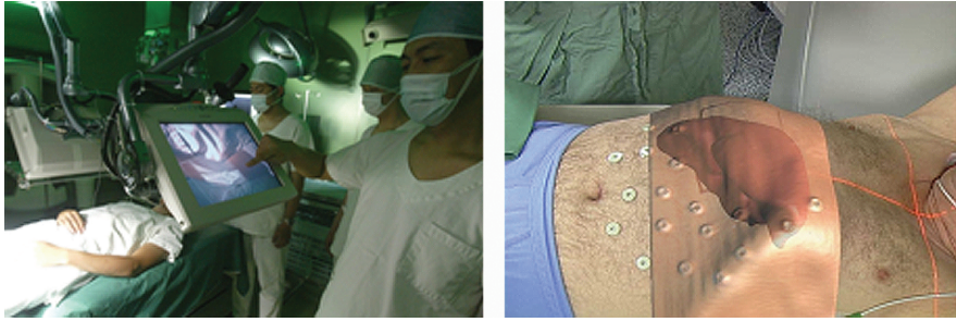
Fig. 4.12. Left: An AR system that combines a video view of the patient with intraoperatively acquired scans of a mobile X-ray C-arm, developed at Jikei University School of Medicine, Tokyo, Japan. Right: Augmented reality guidance for liver punctures with a prototype of a screen-based video AR system developed at IRCAD University Hospital, Strasbourg, France (left picture from Hayashibe et al. 2005 and right picture from Nicolau et al. 2005a, with kind permission of Springer Science and Business Media)
