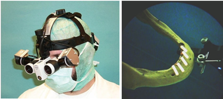
Fig. 4.5. Left: The Varioscope AR , a head-mounted operating microscope with AR visualization, developed at the AKH, Vienna, Austria. Right: Augmented view through one of the oculars, for the scenario of endosteal implant insertion (left picture Birkfellner et al. 2002, © 2002 IEEE; Pictures courtesy of Wolfgang Birkfellner)
