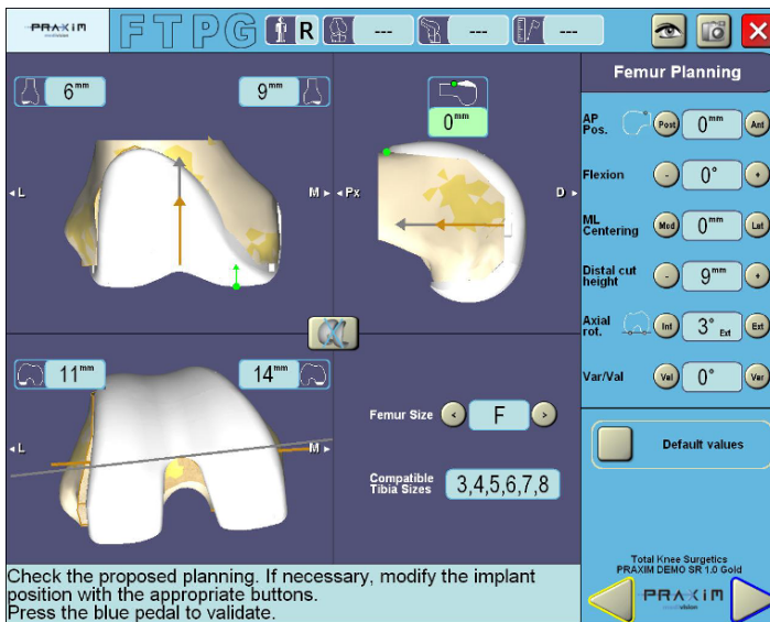
Fig. 12.6. Screenshot from Praxim-Medivision Total Knee Surgetics (TKS) image-free navigation application, based on bone-morphing algorithm. Used with permission.
