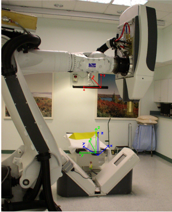
Fig. 16.20. Coordinate systems in the CyberKnife room. The robot, patient, and the Synchrony camera all have separate coordinate systems associated with them that are displayed in different colors.
