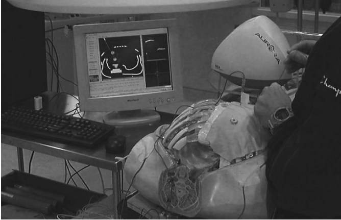
Fig. 13.6. Electromagnetic navigation system and GUI in phantom tests at Georgetown. Reprinted with permission from Banovac et al. [2005]
