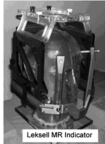
Fig. 16.14. MR indicator – N shaped fiducials as shown on axial scans (Courtesy of Elekta Instrument Inc., Norcross, Georgia)
