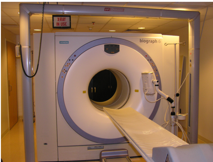
Fig. 9.8. Photograph of a combined CT/PET scanner. Nearly all PET scanners sold today are this type of combined unit. The scanners are arranged in tandem inside a single housing, so that the patient bed can easily move the patient from one scanner to the other. In this case, the CT scanner is on the proximal end of the gantry, and the PET scanner is on the distal end of the gantry
