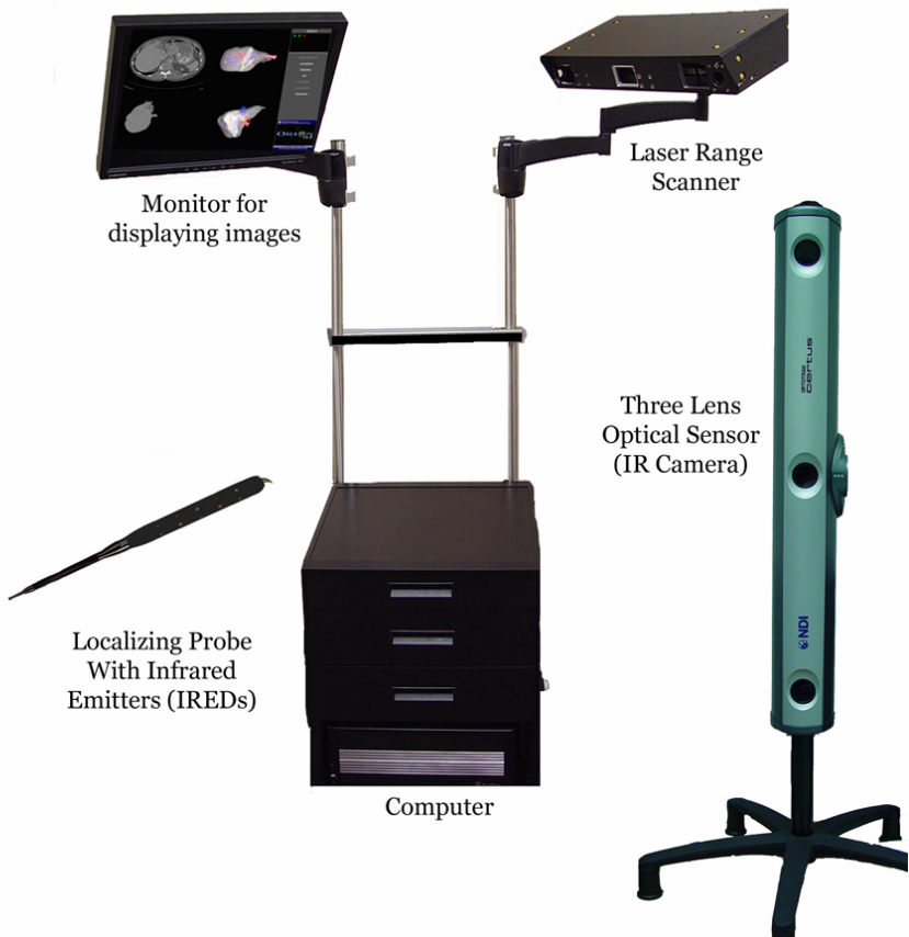
Fig. 13.9. Image-guided liver surgery technology platform under development by Pathfinder Therapeutics Inc. (Nashville, TN). All the components of the system are connected to one central computer located in the bottom of the mobile cart. The three lens optical sensor detects the infrared light and determines the physical position of the probe. The monitor then displays the appropriate images of the organ using data acquired by the laser range scanner and the current probe location. Figure courtesy of Pathfinder Therapeutics Inc.
