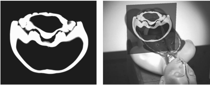
Fig. 4.1. Left: A cross-sectional CT image of a “patient.” Right: Augmented view of the patient with the CT image appearing at the location of the actual anatomy (figures are from Sauer et al. 2000, © 2000 IEEE)
