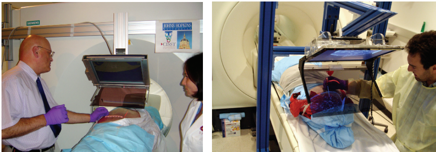
Fig. 4.16. Tomographic overlay systems for percutaneous therapy inside a CT or MRI scanner developed at CISST Lab at Johns Hopkins University. Left: The prototype system with monitor and half-silvered mirror attached to the CT gantry during a cadaver needle placement experiment. All observers see the 2D cross-sectional CT image in the same correct position. A marker is attached to the needle, indicating the length of the needle that has to be inserted to reach the target at the correct depth. Otherwise, the needle is not being tracked, and its actual position inside the patient can only be assessed with a CT control scan. Right: The overlay system constructed around an MRI scanner bed guiding a needle placement procedure (pictures courtesy of Gabor Fichtinger and Gregory Fischer)
