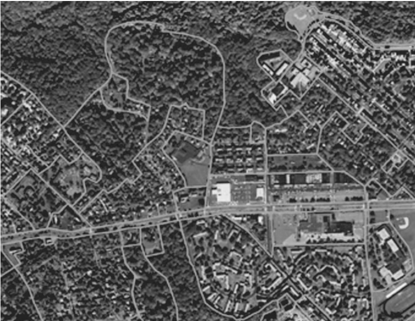
Fig. 1 Patchiness in the Rognel Heights neighborhood of Baltimore, Maryland. The spatial heterogeneity of urban systems presents a rich substrate for integrating ecological, socioeconomic, and physical patterns using Geographic Information Systems. The patch mosaic discriminates patches based on the structures of vegetation and the built environment. The base image is a false color infrared orthorectified photo from October 1999. (M.L. Cadenasso, S.T.A Pickett & W.C. Zipperer, unpublished data.)
