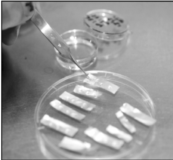
Fig. 15.3 Papaya shoot tips placed in drops of 100% PVS2 on foil strips prior to plunging in liquid nitrogen
