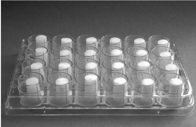
Fig. 8.3 To expose the cells to different solutions without removing them from the multiwell plate commercially available sterilized and dried filters for homemade cigarettes are used. To draw off the old solution a cigarette filter is placed gently in an upright position into each well of the titerplate using a forceps. To regain those cells adsorbed to the bottom of the filter scrape off cells on the edge of the wells
