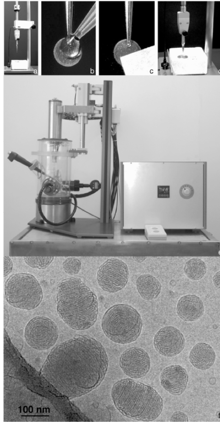
Figure 11.8. Illustration of sample preparation for cryo-TEM imaging. Parts (a)–(d) show specimen preparation for sample freezing; (e) shows plunge freezing apparatus with temperature and humidity control; and (f) a typical image obtained by cryo-TEM. Copyright © 2006 Nestec Ltd.
