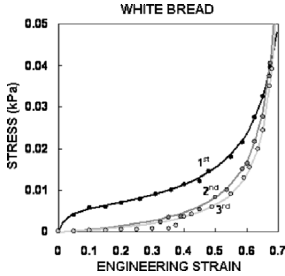
Figure 10.5. The stress–strain relationships of a bread crumb in successive compression–decompression cycles. Notice the disappearance of the shoulder in the second and third cycles, which is probably an indication of closed cells rupture. After Peleg et al. (1989).
