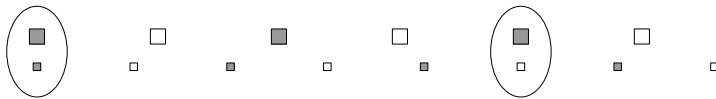
Fig. 13.10. The cross section of a two layer grid with the line pitch of the upper layer a fractional multiple ( 5/4 in the case shown) of the line pitch in the bottom layer. Both effects illustrated in Fig. 13.8 occur at different locations (circled). The ground lines are white colored, the power lines are grey colored.
