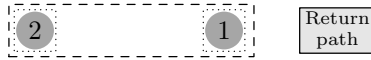
Fig. 10.2. A cross-sectional view of two parallel current paths (dark gray) sharing the same current return path (light gray). The path closest to the return path, path 1, has a lower inductance than the other path, path 2. The parallel paths can be either two physically distinct lines, as shown by the dotted line, or two different paths within the same line, as shown by the dashed line.
