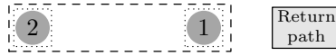
Fig. 2.11. A cross-sectional view of two parallel current paths (dark gray) sharing the same current return path (light gray circles). The path closest to the return path, path 1, has a lower inductance than the other path, path 2. The parallel paths can be either two physically distinct lines, as shown by the dotted line, or two different paths within the same line, as shown by the dashed line.
