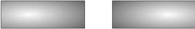
Fig. 2.9. Proximity effect in two closely spaced lines. Current density distribution in the cross section of two closely spaced lines at high frequencies is shown in shades of gray. Darker shades of gray indicate higher current densities. In lines carrying current in the same direction (parallel currents), the current concentration is shifted away from the parallel current. In lines carrying current in opposite directions (antiparallel currents), the current concentrates toward the antiparallel current, minimizing the circuit inductance.
