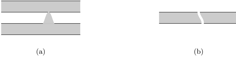
Fig. 4.1. Electromigration induced circuit faults. (a) Line extrusions formed due to metal accumulation can short circuit the adjacent line. (b) The voids formed due to metal depletion increase the line resistance and can lead to an open circuit.
