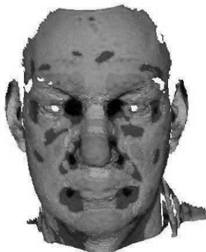
Fig. 11.5. Curvature-sign based labeling of pixels in a 3D image of a face.
