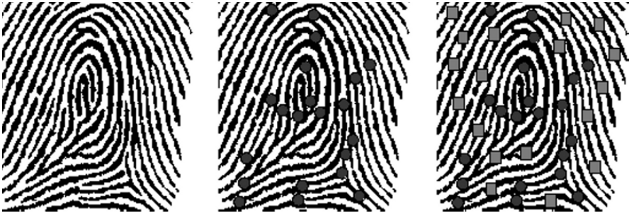
Fig. 19.5. Schematic diagram of the biometric encryption scheme of [8]. Left: a raw fingerprint image is enrolled. Middle: minutiae points (circles) are used to encode the value of a polynomial representing the secret. Right: chaff points (squares), sufficiently far from minutiae, are used to encode random values of the polynomial.
