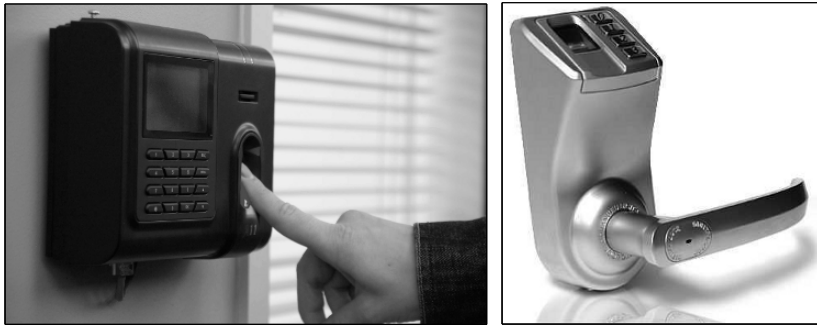
Fig. 23.3. The first picture shows a biometric-enabled stand-alone physical access control system for room entry. The second picture shows a biometric-enabled stand-alone door lock.
