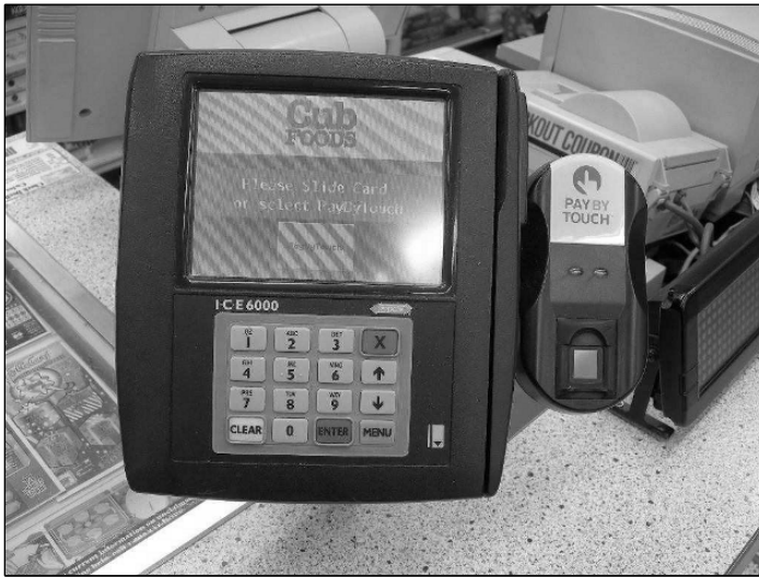
Fig. 23.8. A Point-Of-Sale terminal with integrated fingerprint reader. In this commercial application, the customers do not need to carry a credit/loyalty card to make payment for merchandise; they are authenticated by fingerprints against their account number entered through the keypad.
