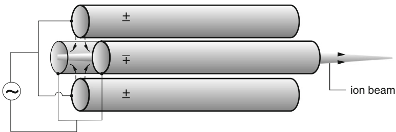
Figure 12.3 The Paul high-frequency ion mass filter
