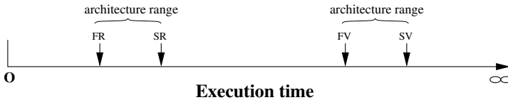
Fig. 5. The required order of execution times for a Benchmark for different configurations. Given some configuration information, FR is the fastest real machine, SR is the slowest real machine, FV is the fastest real machine running the fastest VMM, and SV is the slowest real machine running a VMM.
