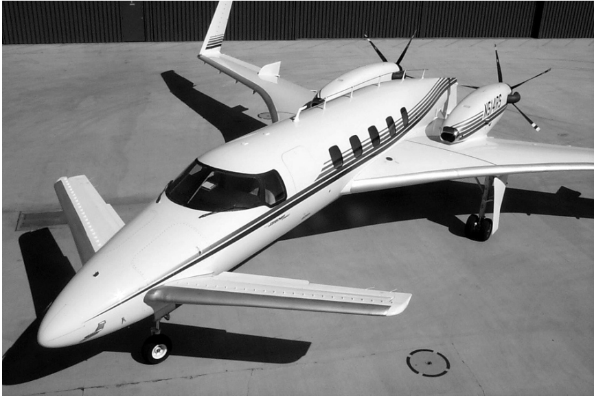
Fig. 1.3 The almost all-composite Beechcraft Starship (courtesy of Robert Scherer, http://www.bobscherer.com )
