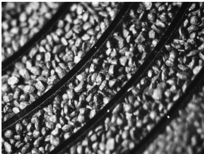
Fig. 5. Encapsulated silicon spiral column packed with a commercial gas chromatography stationary phase [17]. Reprinted with permission
