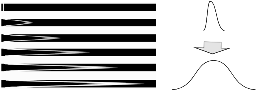
Fig. 9. Poiseuille flow transporting an initially well-localized concentration tracer through a channel ( left ) and evolution of the cross-section averaged concentration ( right ). Irrespectively of the initial concentration profile, the final distribution is a Gaussian
