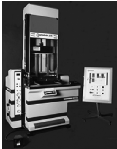
Fig. 9.4. Lead-free vertical HASL machine (Source: Cemco-FSL)
