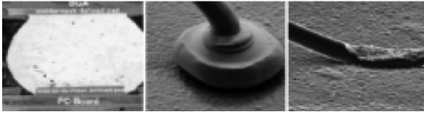
Fig. 9.20. The Ni/Pd/Au finish is suitable for soldering as well as gold and aluminum wire bonding (Source: Atotech)
