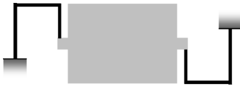
Figure 2.52 Top view of a microaccelerometer with two fishhook springs
