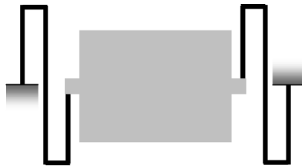
Figure 2.25 Top view of a microaccelerometer with basic serpentine springs
