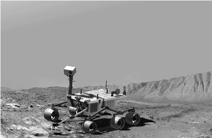
Figure 102: Artist's impression of NASA/JPL Mars Science Laboratory (MSL). MSL will be larger than the MER rovers, be able to travel over 10 kilometers from its landing site, and look for evidence of biology on Mars. [Credit: NASA/JPL]
