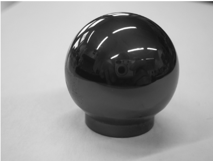
Fig. 3 DLC-coated femoral head of a hip joint
