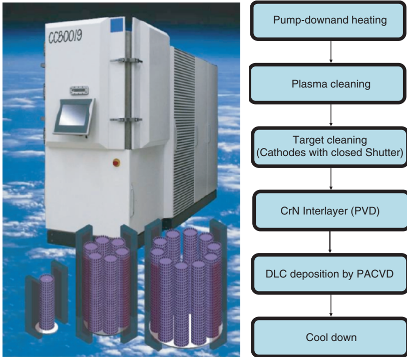
Fig. 2 (Left) Different batch sizes for cutting inserts for a CC800/9 coating unit and (right) process-flow diagram of a typical DLC process
