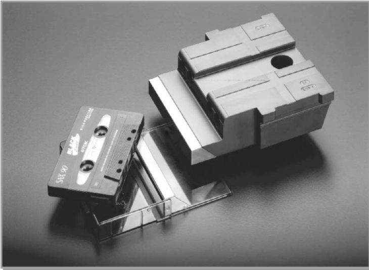
Fig. 7 DLC-coated plastic injection mold for manufacturing of polystyrene-covers for magnetic tapes; maximum coating temperature 200°C
