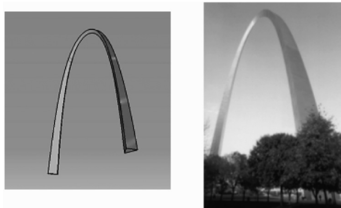
Figure 1 - Comparison of the Solid Model from the CATIA Screen to an Actual Photo. The CATIA image is an infinite perspective. The photo has some distortion due to the fact that it was taken with a 100-mm lens.
