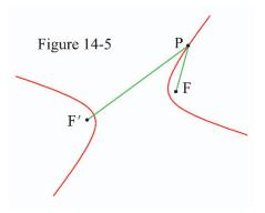
where FF' is the *interfocal separation*, the distance between the two foci, equal to 2*ka*. The two parameters of the hyperbola (sometimes called its *semiaxes*) are *a*, defined in 14:14:1 and *b*, given by
