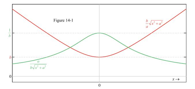
regarded as positive throughout the chapter. The adjectives "vertical" and "horizontal" will be used to distinguish between the  $(b/a)\sqrt{x^2 + a^2}$  and  $(b/a)\sqrt{x^2 - a^2}$  functions, in recognition of their graphical orientation. These two functions are said to be *conjugates* of each other.
