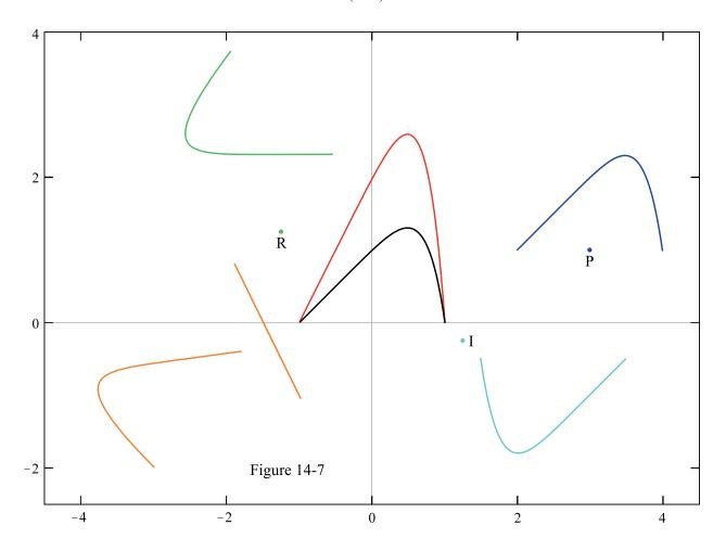
*Reflection in the line* bx+c implies that, from each point on the original graph, a perpendicular is dropped onto the line and then extrapolated to a new point that is as far from the line as was the line from the original point. The formulas governing this operation, are
