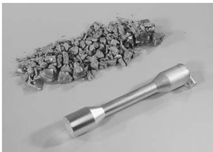
Fig. 9 Total disintegration of a Sn-0.5Cu test piece after prolonged exposure at -18^{\circ}\text{C}
