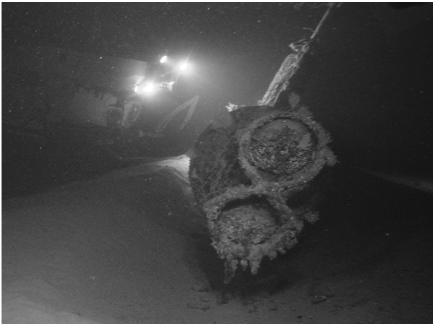
FIGURE 13.2. Two type-97 "mini" Long Lance torpedoes still are loaded in their forward tubes. Note the scoured area beneath the bow of the sub (Photo courtesy of HURL).
