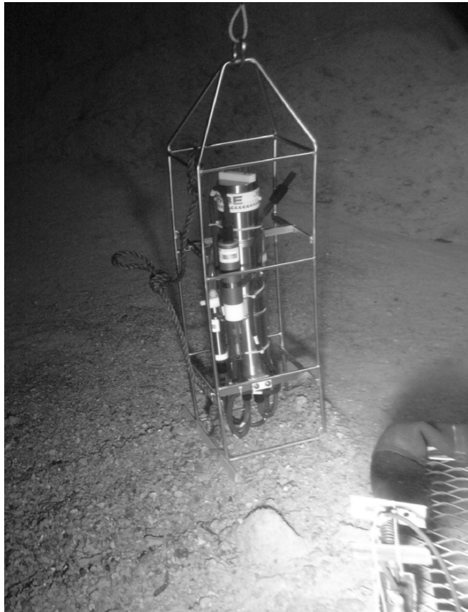
FIGURE 13.3. Science at the heritage resource site: SeaBird ocean profiler collecting various parameters to initiate long-term study and preservation management plan (Photo courtesy of NOAA NMSP).
