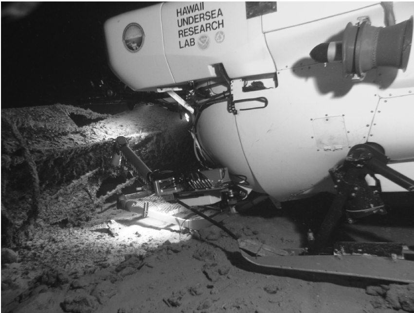
FIGURE 13.5. HURL's Pisces IV conducting survey work near the stern dive planes of the Ko-Hyoteki (Photo courtesy of NOAA NMSP).
