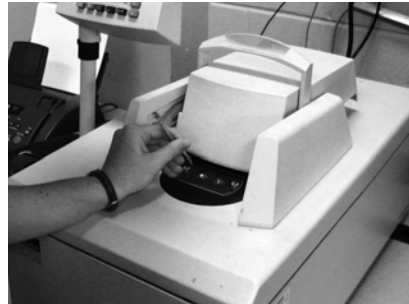
(b) SMA sample loaded into a DSC system.
