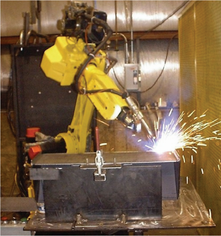
Fig. 9.1 Fanuc Arc-Mate 120-i Robot Welding Cell ( Courtesy-Burns Machines )
