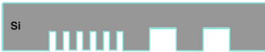
(iii) Deposition of the protective thin film after removal of the \text{SiO}_2
