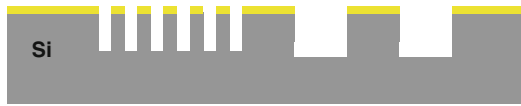
(ii) Silicon DRIE etch using \text{SiO}_2 as hard mask to form HAR structures
