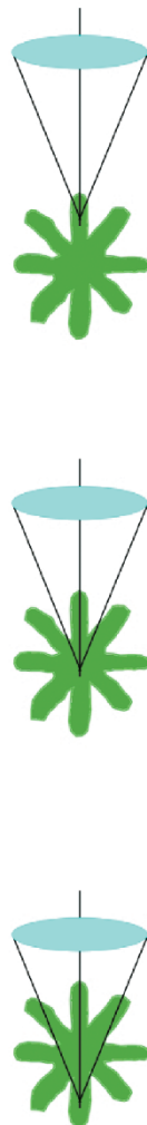
FIGURE 8.47. Self-shadowing phenomenon in epi-fluorescent mode. As the specimen attenuates both the excitation and the detected fluorescence, intensity is lower for structures located in deeper parts of the specimen. This phenomenon is particularly pronounced when the specimen is very densely stained or pigmented. (A, B, C) Epi-fluorescent confocal images of a living alga, Closterium . Three images were obtained under the same conditions. (A) Optical section showing chlorophyll autofluorescence near the top of the specimen, (B) from the middle of the specimen ( 35\ \mu\text{m} from the top of the surface) and (C) from the bottom of the specimen ( 70\ \mu\text{m} from the top of the surface). Note the reduction of the fluorescent signal (particularly in the center of the specimen where there is maximum shading).
