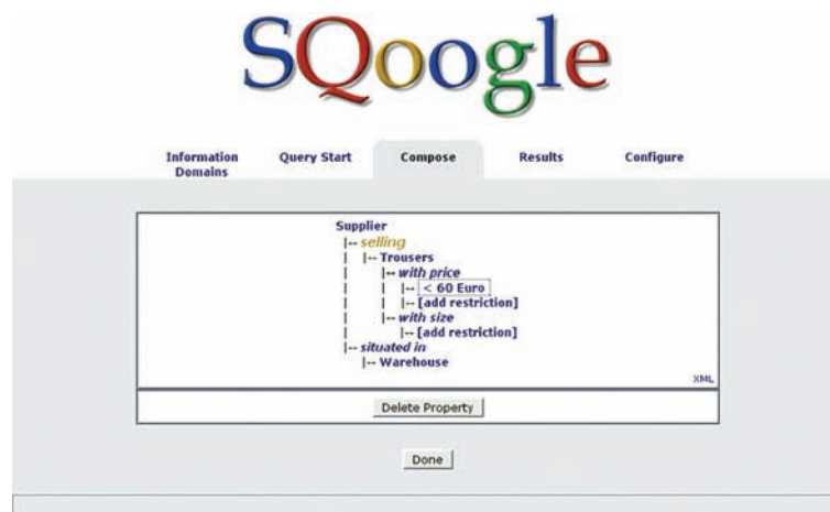
Ontology Visual Querying. Figure 1. Visual query expression in SQoogle. The query is to select suppliers that sell trousers that cost less than 60 euros, where the supplier is situated in a warehouse.
