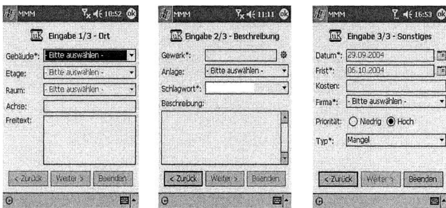
Figure 5 - Screen-shot Mobile Application for Error and Omission Management ( Ort=Localization, Beschreibung=Specification, Sonstiges=Costs & Deadlines )
