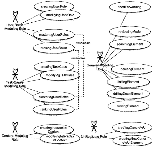
Fig. 55. User Role Model for a Usage-Centered Design Tool (full model omitted for brevity).
