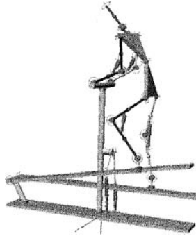
Fig. 33. Operator's position on the treadle pump
