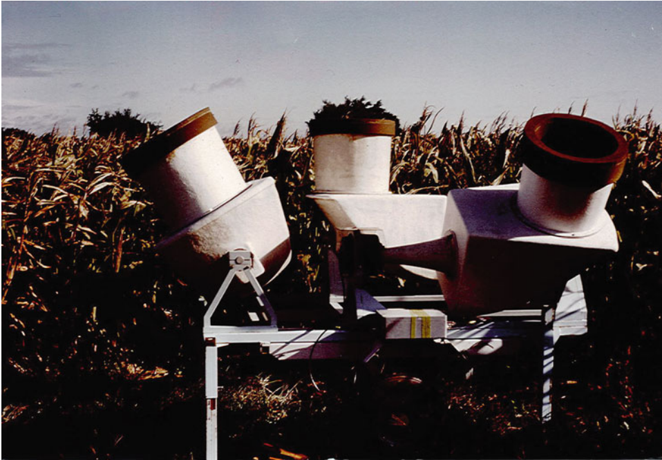
Acoustic Radiation, Figure 1 Realization of a three offset antennas for a 6 kHz minisounder. One antenna is vertical and two others are slanting . One distinguishes compression chambers as acoustic sources and the horns and antennas parts ( parabolic portion + circular aperture covered by acoustic foam ).
