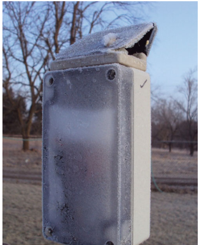
Emerging Technologies, Sensor Web, Figure 4 Sensor nodes based on solar panels and rechargeable batteries typically have problems associated with sub-zero temperatures.
