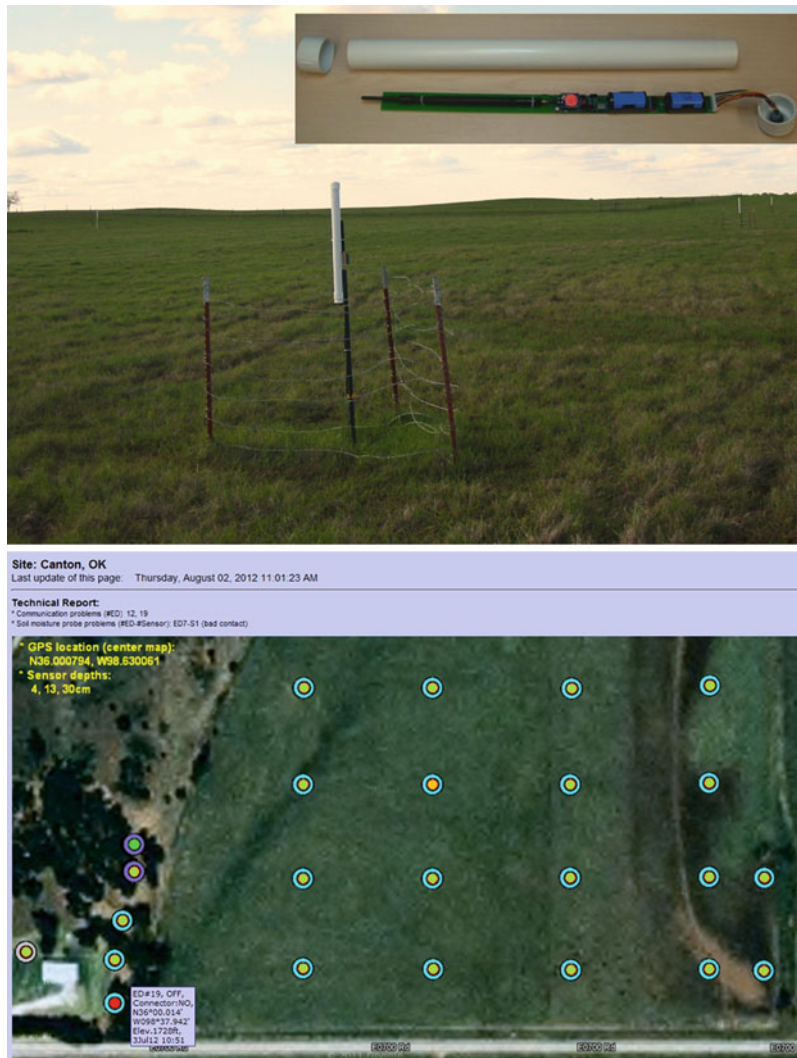
Emerging Technologies, Sensor Web, Figure 5 A Ripple-2 node powered by non-rechargeable batteries ( top ) installed in SoilSCAPE field locations such as Canton, OK, USA ( bottom ).
