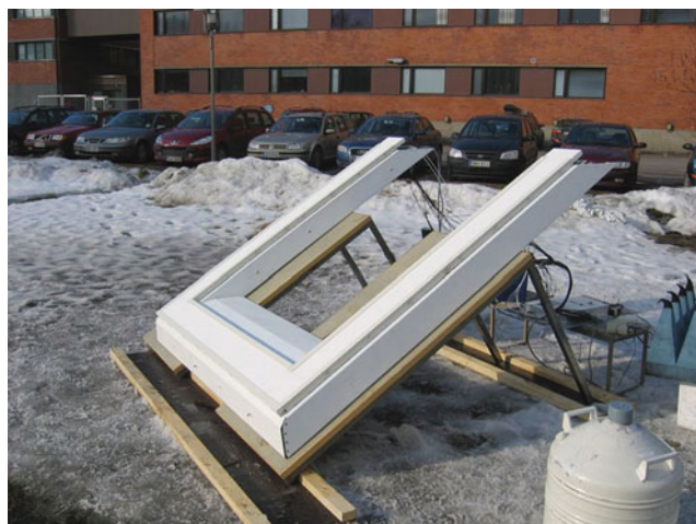
Microwave Radiometers, Interferometers, Figure 2 Helsinki University of Technology's two-dimensional airborne interferometer (HUT-2D) (Courtesy Martti Hallikainen, TKK).
