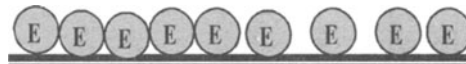
Fig. 1. Enzyme layer resulting from adsorption of enzyme on a surface and binding due to van der Waals or ionic forces. Covalent coupling results also in a monolayer-coverage, if cross-linking of enzyme molecules is avoided
