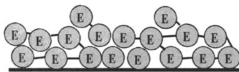
Fig. 8: Enzyme adsorbed on a surface followed by cross-linking of proteins with bifunctional reagents. The thickness of the layer depends on the amount of adsorbed protein
