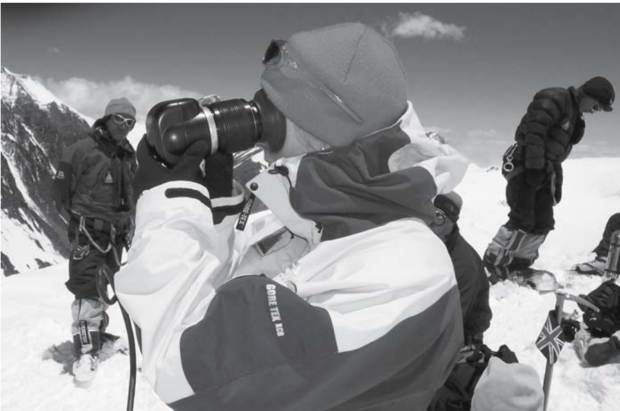
Figure 9. Measuring color vision with a prototype instrument at Everest north col (7100m).
