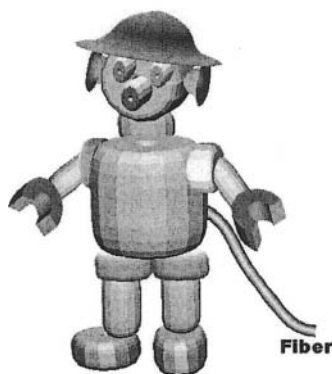
Figure 14. (Left) Robot can be driven by fiber laser. The right figure shows the assistant robot that uses only 50W laser (Size 80×60×100cm. Courtesy of Yukio Takeda, Tokyo Institute of Technology).
