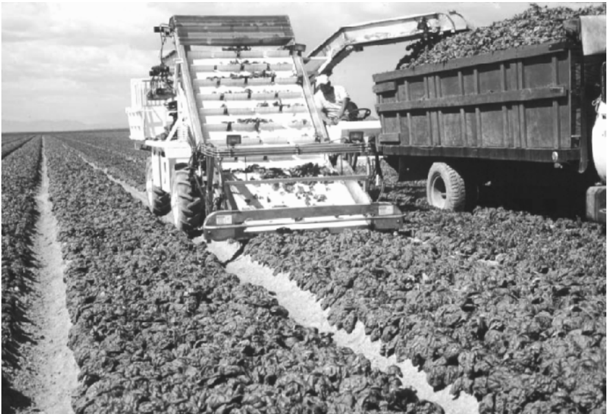
Fig. 6. Band saw harvester cutting fresh market spinach.
