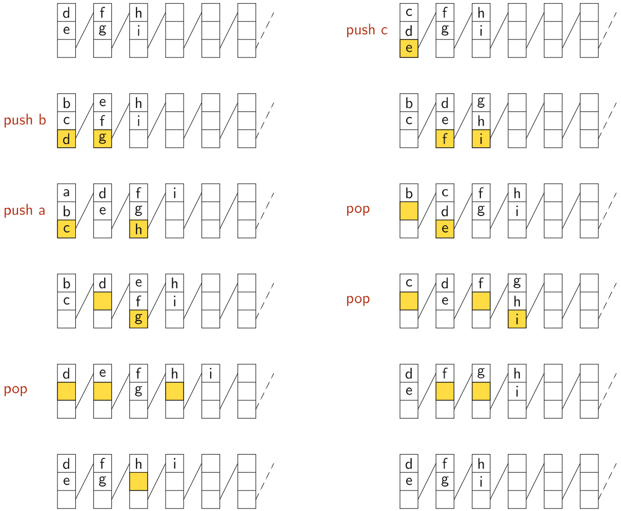
Cellular Automata and Language Theory, Figure 6 Principle of a pushdown store simulation. Subfigures are in row-major order
